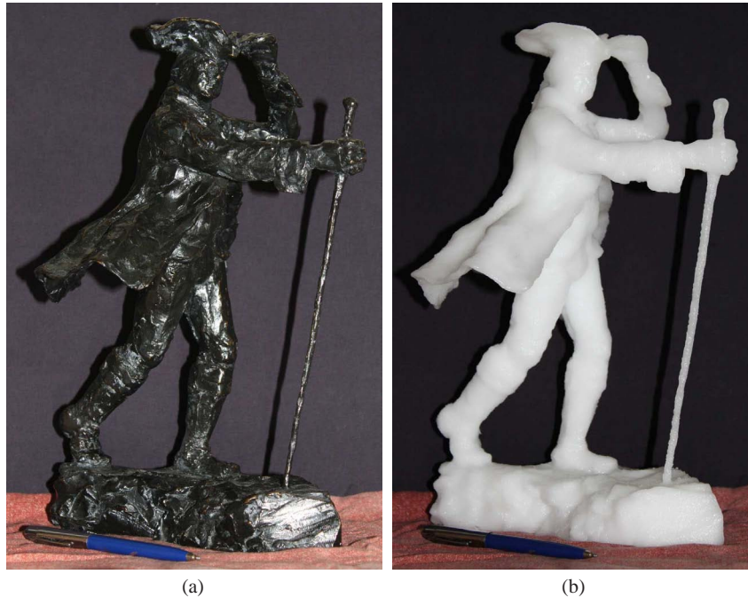
Fig. 5 James McGill statue, 306 mm high: (a) Original bronze statue; (b) Ice statue, built on its side, with the Cobra 600 RFP system: 852 slices built in 132 hours
