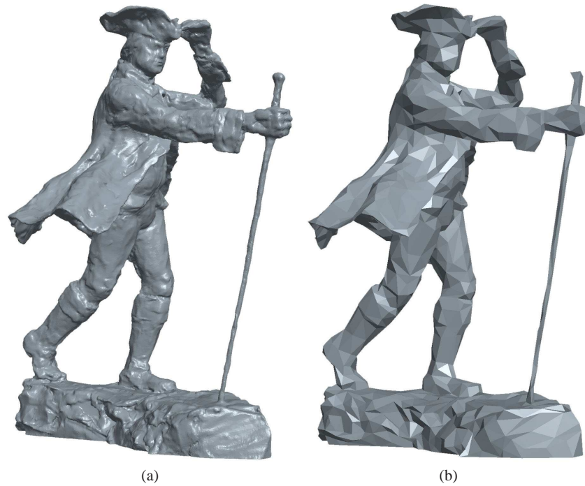
Fig. 1 James McGill STL part: (a) One million facet model; (b) Decimated model with 3906 facets
