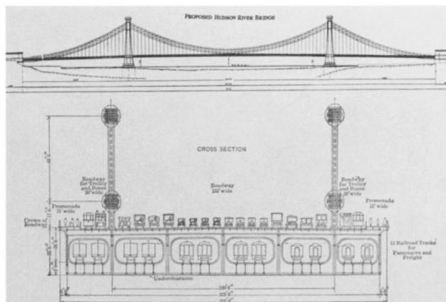
Fig. 5. Hudson River, proposed suspension bridge, G. Lindenthal, 1921. Elevation and section (Steinmann, *Suspension Bridges*, 1929).
