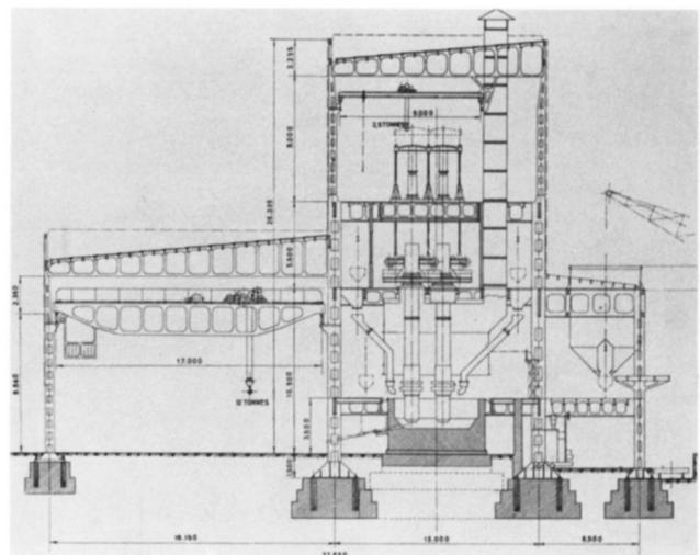
Fig. 10. Savone, new ILVA Steelworks, A. Bozzarelli, 1939. Transverse building section (*L'Ossature Metallique*, March 1940).
